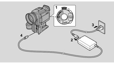
Use the power adapter to provide your camcorder with instant power from a household power socket. Always turn the camcorder off before connecting/removing the power source.
